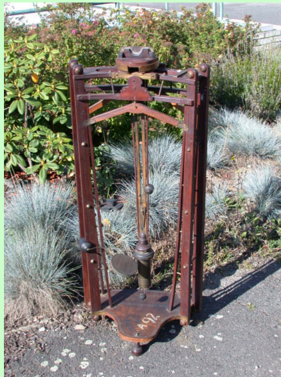
Torso of Carl Kreil's pendulum (seismoscope) constructed in Prague German University around 1849. Now kept in the National Technical Museum, Prague.
