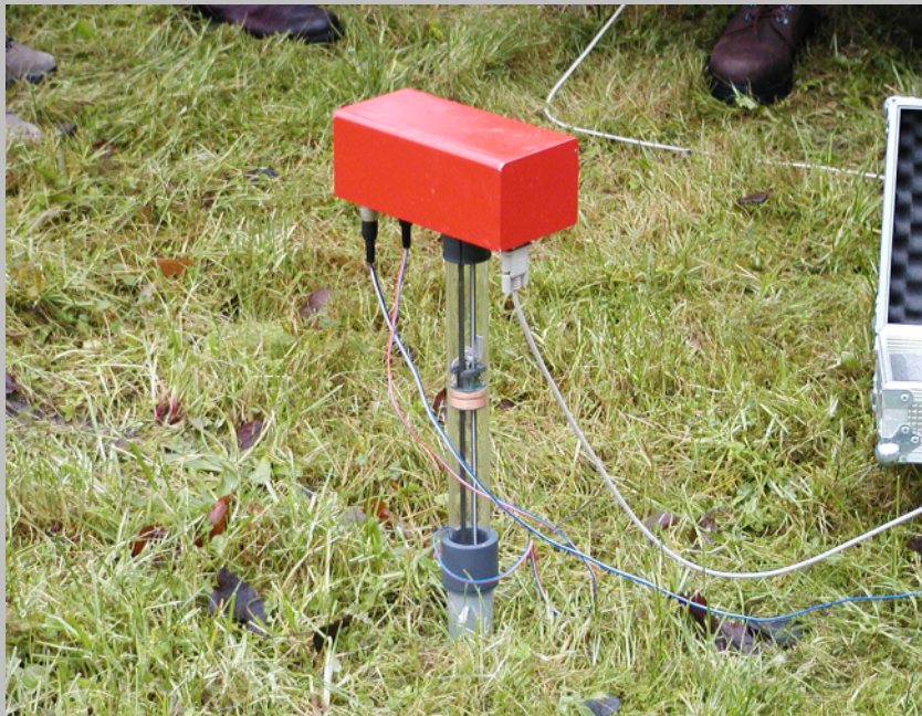
Susceptometer SM400 for real-time measurements of vertical distribution of magnetic susceptibility in soils (developed within EU 5FP Project MAGPROX).
