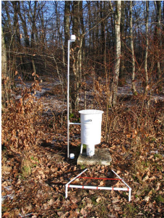
Fig. 3. The borehole climate change station near Slovenian Kostanjevica established in 2003 monitors the air, soil and bedrock temperatures down to the depth of 40 m with a sampling interval of 30 minutes.
