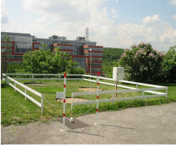
The air-ground temperature monitoring on the campus of the Geophysical Institute at Prague – Spořilov.
