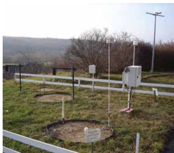
— Figure 2 Air-ground temperature monitoring on the campus of Institute of Geophysics at Prague – Spořilov.
