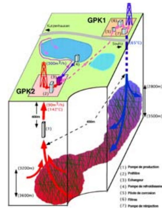
Fig.2. Sketch of the EGS facility Soultz-sous-Forêts at an early stage of its operation (Cuénot, 2010).
