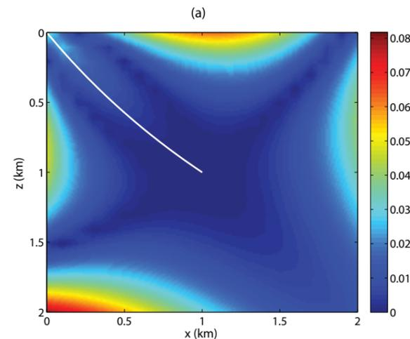
*Accuracy of approximate two-point traveltimes formula. Approximate traveltimes are computed from quantities calculated along the reference ray (white curve). Plot shows a map of deviations of P-wave approximate traveltimes from exact ones in an isotropic model with constant vertical velocity gradient.*
