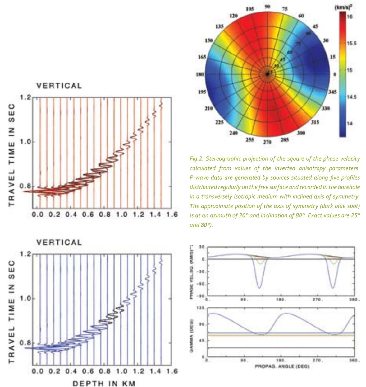
Fig.2. Stereographic projection of the square of the phase velocity calculated from values of the inverted anisotropy parameters. P-wave data are generated by sources situated along five profiles distributed regularly on the free surface and recorded in the borehole in a transversely isotropic medium with inclined axis of symmetry. The approximate position of the axis of symmetry (dark blue spot) is at an azimuth of 20° and inclination of 80°. Exact values are 25° and 80°.
