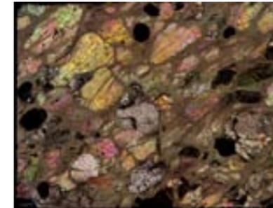
Dynamic recrystallization of garnetiferous peridotite shown in a thin section, polarized light
