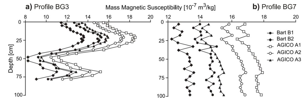
Fig. 1. Mass-specific MS of soil profile BG3 (a) and BG7 (b), measured using Bartington (frequencies B1 = 0.465 kHz, B2 = 4.65 kHz, amplitudes of magnetizing field 80 Am<sup>-1</sup>) and AGICO instrument (frequencies A1 = 0.975 kHz, A2 = 3.904 kHz, A3 = 15.616 kHz, amplitudes of magnetizing field 200 Am<sup>-1</sup>).
