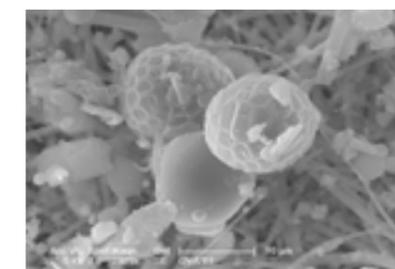
Spherules of industrial origin rich in magnetite ( $\text{FeOFe}_2\text{O}_3$ ) as part of flight ash.
