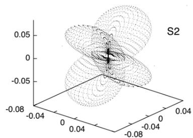
Directivity functions (spreading-free amplitudes at a source) of P (top), S1 (middle) and S2 (bottom) waves generated by an explosive source in an orthorhombic medium. Note that S1 and S2 waves would not be generated if the medium is isotropic.
