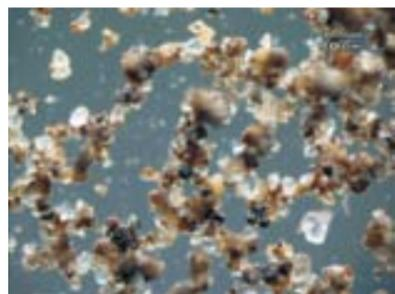
Magnetic extract of topsoil sample from the Ostrava region (N Moravia), with dark spherical magnetite of industrial origin.
