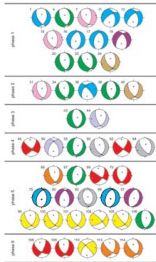
Fig.4: Source mechanisms of 45 micro-earthquakes that occurred during individual stages of the injection experiment (Horálek et al., 2010).
