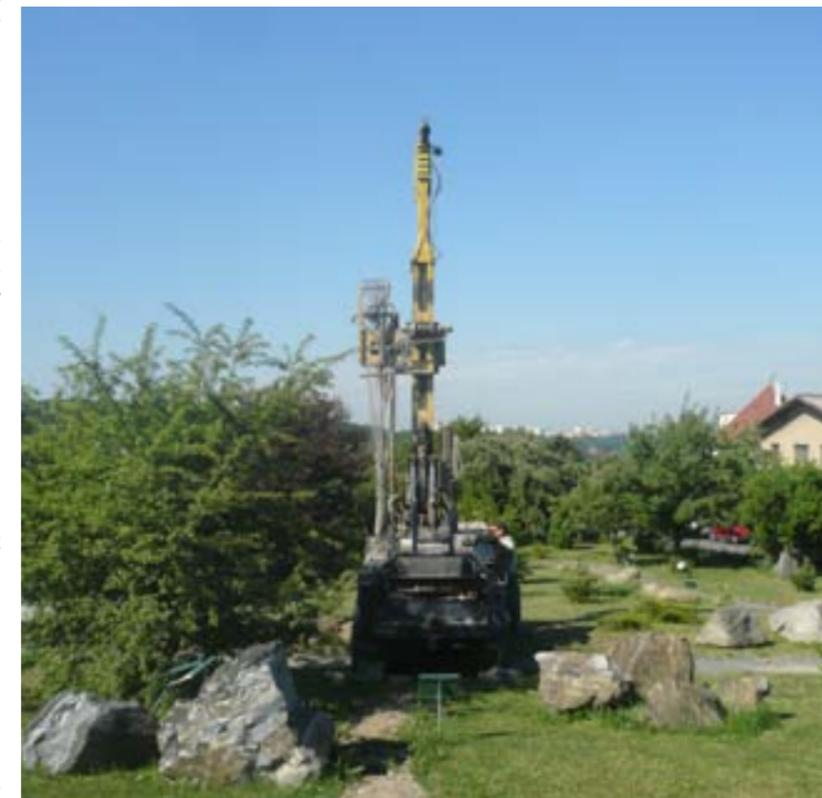
Drilling the borehole for the new geothermal observational site – Spořilov 3, in the Geopark of the Institute of Geophysics, May 2011.
