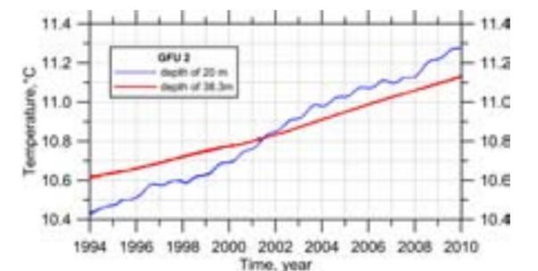
Fig.1. Sixteen year long time series of continuous temperature monitoring at two different depths (20 m and 38.3 m) of the borehole GFU-2 located on the campus of the Institute of Geophysics in Prague. In agreement with the theory, (i) amplitude of the warming propagating from the ground surface downward is larger at 20 m than at 38.3 m, (ii) the seasonal changes fade out between 20 m and 38.3 m.
