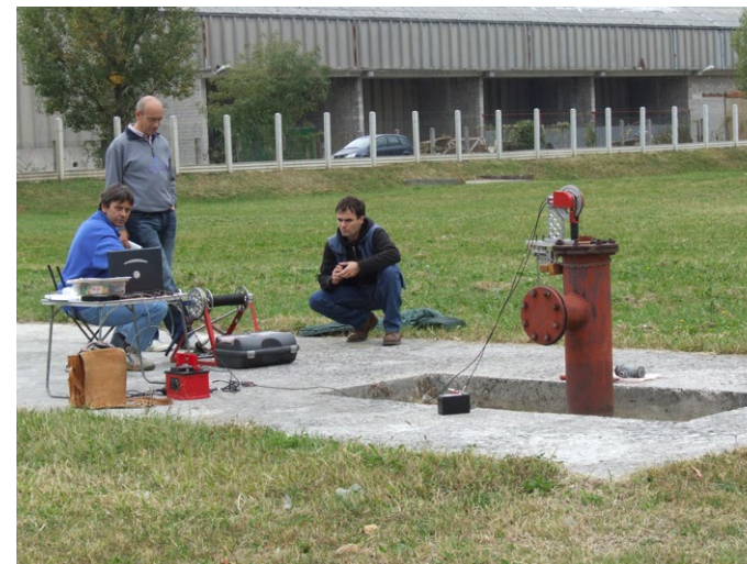
Acquisition of a temperature–depth log on site of one of boreholes studied in Slovenia
