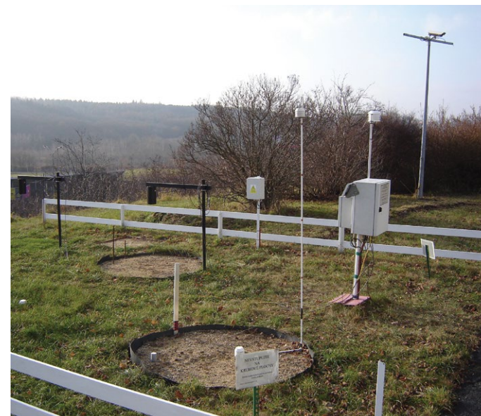
Fig. 9: Air-ground temperature monitoring on the campus of the Institute of Geophysics.
