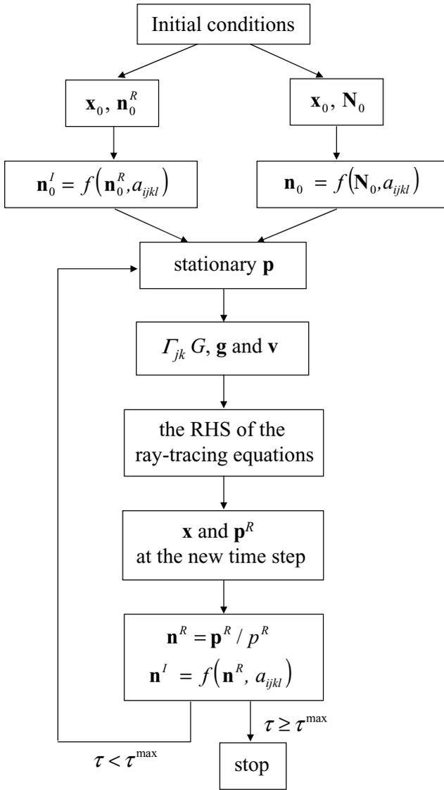
**Figure 1.** A scheme of the numerical procedure for ray tracing in anisotropic viscoelastic media.
