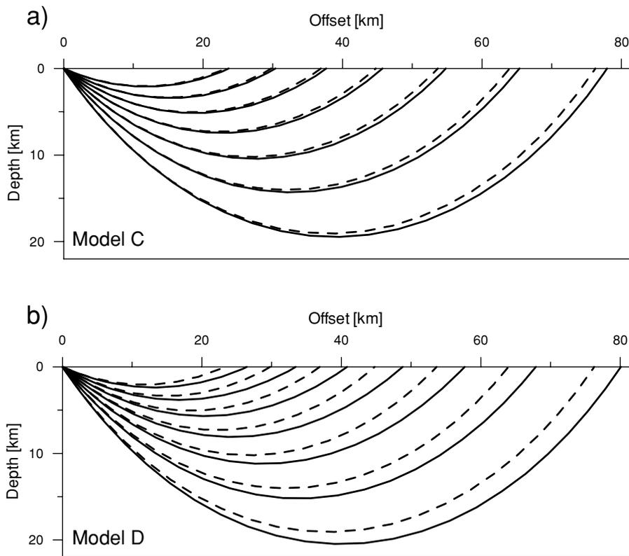
**Figure 5.** Ray fields in models C (a) and D (b). Solid line, rays calculated in the viscoelastic medium; dashed line; rays calculated in the elastic background. For parameters of the media and rays, see the text.
