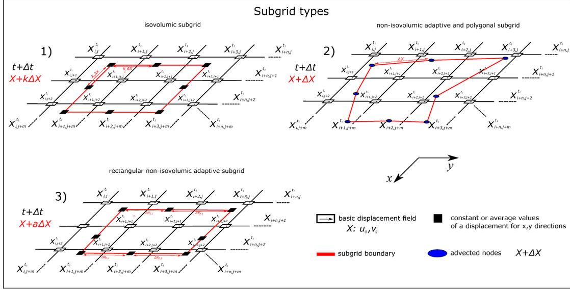
Fig. 31: Types and interpolation strategies for the interrogation subgrids. The three selected subgrid types are described in the text. Red lines show the shapes of the subgrids. The black rectangles at subgrid boundaries represent the constant or average values of displacement, while the blue ellipses correspond to subgrid boundary nodes with individual displacement in both directions.
