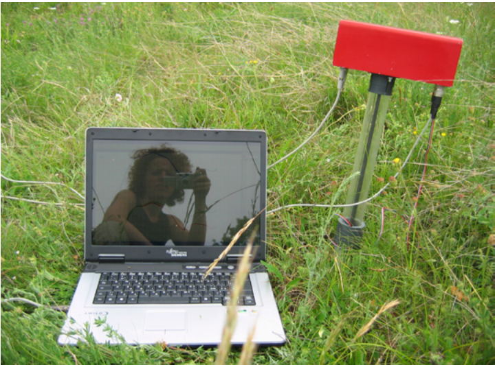
Fieldwork in the Massif Central, France, with Hana Grison in action conducting in situ measurements of the vertical distribution of magnetic susceptibility using an SM 400 kappameter (Photo: H. Grison). Grison et al. (2016) examine the chemical and magnetic attributes of soils (andosols) developed on volcanic rocks in the French Massif Central, with the aim of identifying a magnetic signature of pedogenic development.
