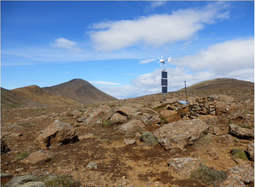
Fig. 3. REYKJANET: Station FAF (Fagradalsfjall) is of key importance for Reykjanes seismic observations. The seismic activity has been growing under the Fagradarsfjall volcano since 2017 reaching a magnitude M_w=5 in earthquake swarms of 2020.
