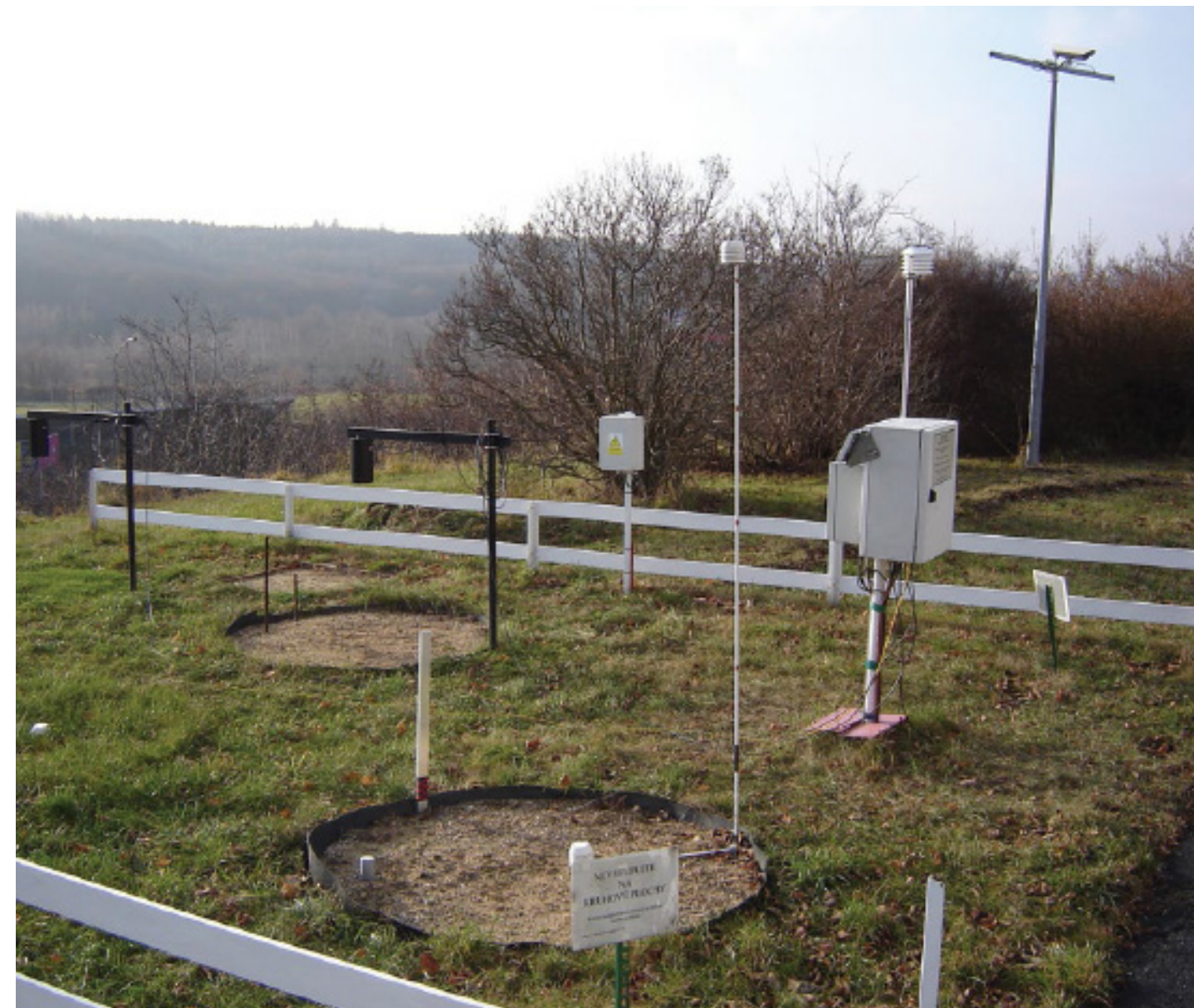
Air-ground temperature monitoring on the campus of the Institute of Geophysics.
